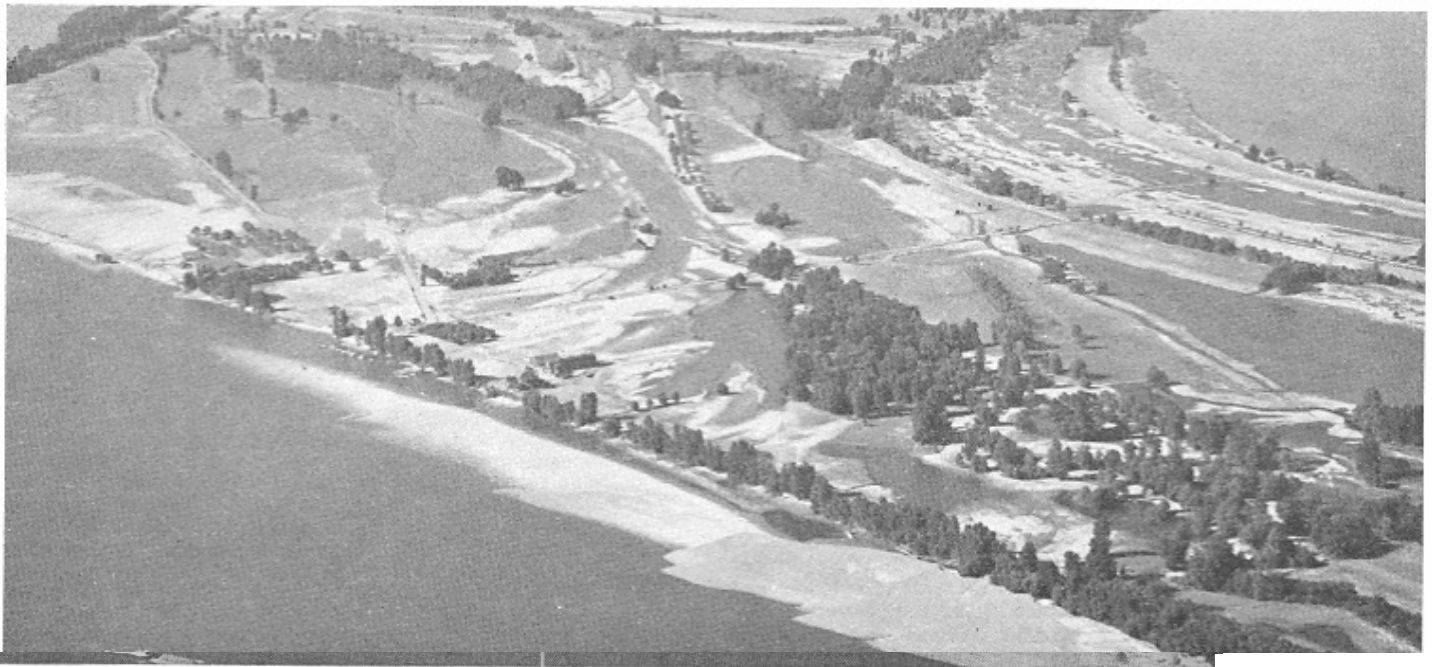
Figure 11.-Deposition of sand on Newberg silt loam, 0 to 3 percent slopes, middle ground, that resulted from flooding by the Columbia River. The sandy soil along the river in the right foreground is an area of Riverwash. This area is 3 miles downriver from Vancouver.
